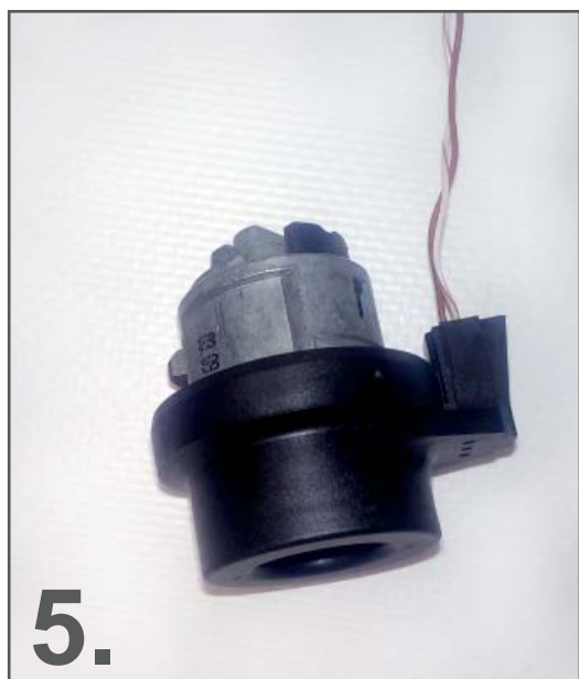
Connect two gold pins into reading coil. You can commute them.
